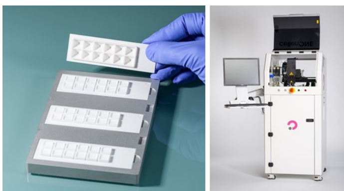
Figure 1. Pictures of the proteoCHIP 12*16 and the cellenONE® single cell isolation and picoliter dispensing platform. (left panel) proteoCHIP 12*16. Three nanowell part (bottom) placed in their dedicated holder. One funnel part (top) used for pooling each sets of multiplexed sample and direct injection into the autosampler. (right panel) Illustration of the cellenONE®.
